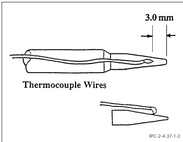
**Figure 2 Thermocouple Placement**
