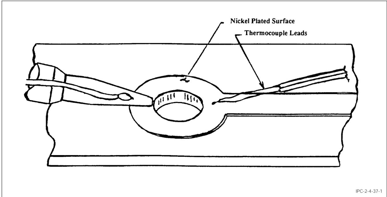
**Figure 1 Placement of Thermocouple Leads**
