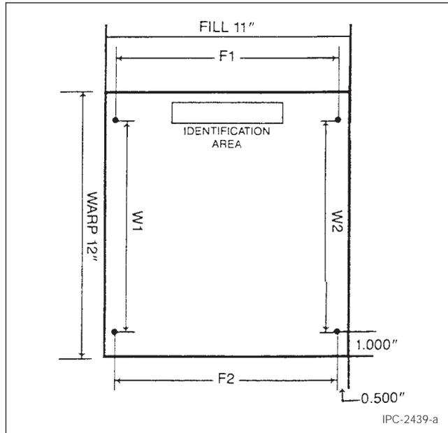
**Figure 1** All dimensions are in inches. Four measurements are required as indicated. Locate measuring points approximately 12.7mm [0.500 in] from each edge in the fill direction, and 25.4 mm [1.00 in] from each edge in the warp direction.
