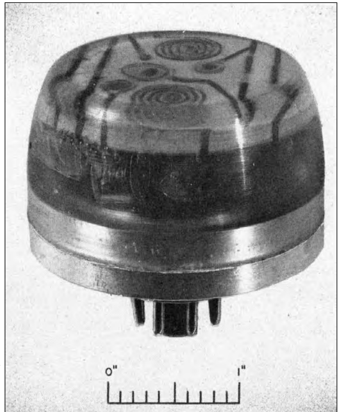
FIGURE 38. Printed plug-in unit encased in NBS casting resin.
