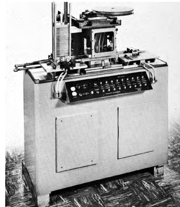
Two types of machines for automatic terminal and lug insertion in high production TV panel manufacture.
