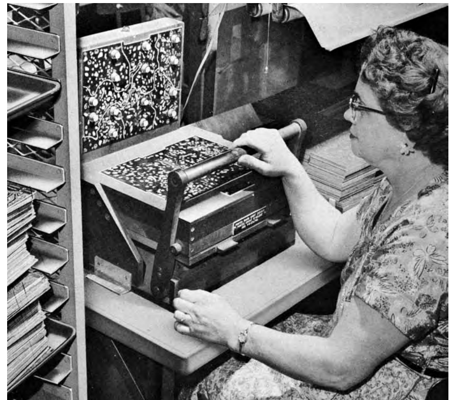
Reliability is assisted by equipment such as this hipot testing fixture for complex panels. Using spring loaded test prods to contact adjacent circuits, the general area of a short circuit is located by indicator lights.
