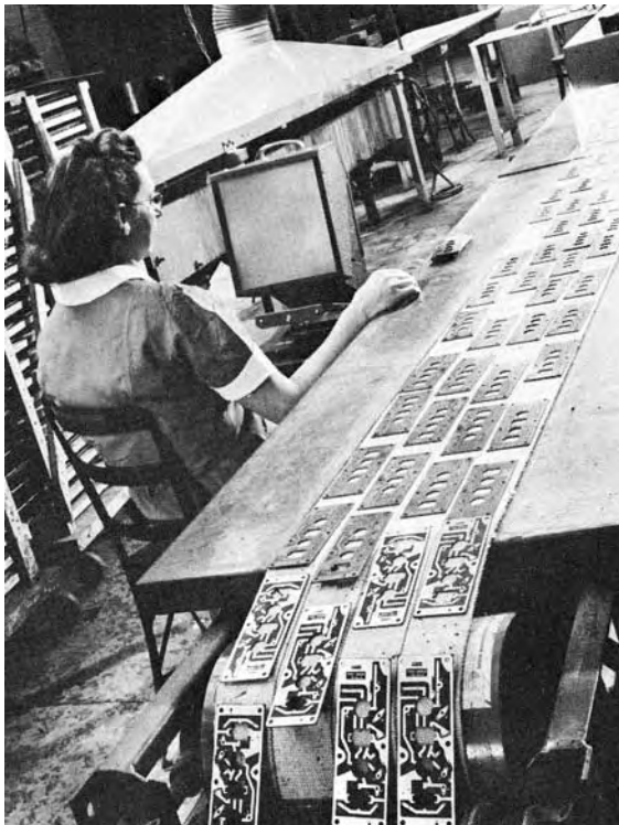
Conveyorized processing and inspection of etched circuit panels.
