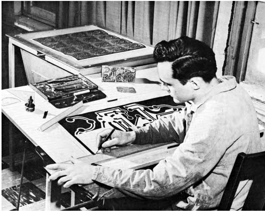
Drafting of master black and white printed conductor layout. Drawings should be several times actual size for best results in reproduction.
