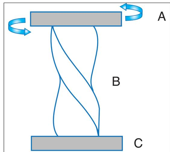
**Figure 3 Torsion Test Setup**
